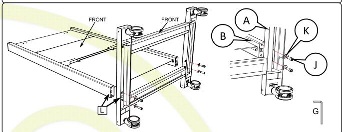
Assemble the handle to the frame ( 5 mm)
