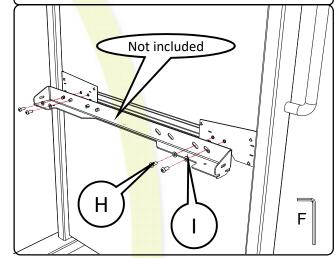
Mount the BalanceBox®650 on the wall bracket and assemble the screws at the top(● 5 mm)
