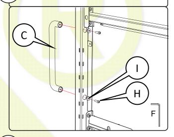
Mount the BalanceBox®650 wall bracket to the frame as shown(● 5 mm)
